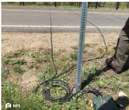
Image 2: Road tube counters at the Grand Lake Entrance Station. Road tubes are attached to counter.
