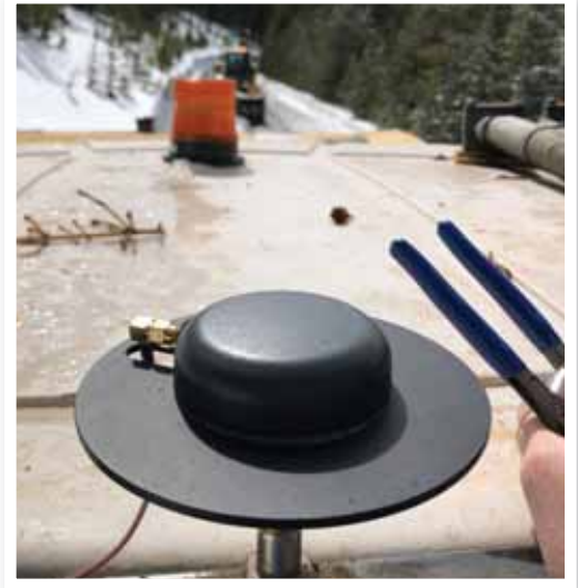
To help operators navigate Trail Ridge Road during plowing operations, the Arrow Gold's antennae sits on the top of the snowplow.
