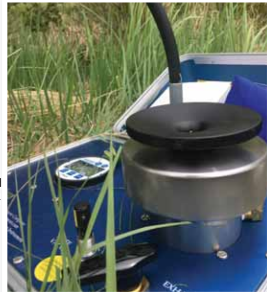
The main scientific device Isabel used to measure plant water status in the field. This instrument — the Scholander Pressure chamber — is a classic piece of plant physiological equipment. It assesses how much pressure is required to force water out of a small branch, and taken at peak temperature and light conditions, it provides an indication of how much water stress a plant is experiencing — more pressure means higher stress.
