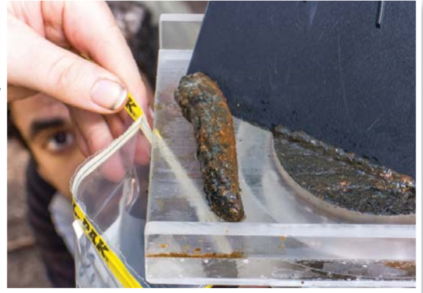
Sediments collected from the center of the lake are often sectioned in the field as soon as possible. The core collected from Pipit Lake was sectioned at 0.25 cm increments which will offer high-resolution data for environmental and climatic change. The sediment in the image clumped together nicely due to the high clay content present and made the sediment easier to bag for future analysis.
