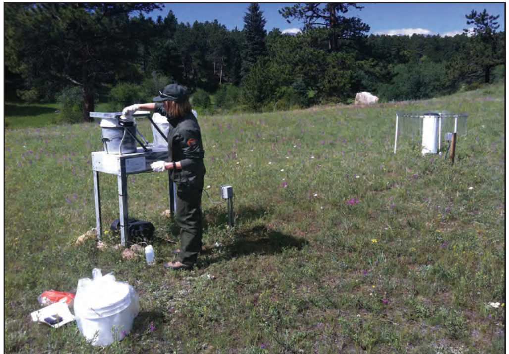
National Atmospheric Deposition Program (NADP) sites like this one in the park (deposition buckets and a rain gauge), are sampled weekly to measure nitrogen deposited by rain and snow.
